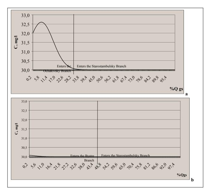
Figure 2. Concentration Ranges for Suspended Substances under Option 1 at the Gauging Stations No. 1 (a) and 2 (b)
