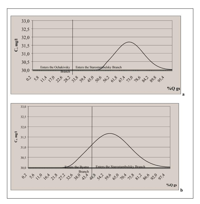
Figure 4. Concentration Ranges for Suspended Substances under Option 3 at the Gauging Stations No. 1 (a) and 2 (b)
