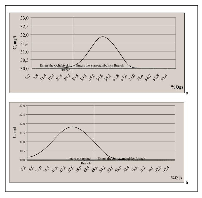
Figure 5. Concentration Ranges for Suspended Substances under Option 4 at the Gauging Stations No. 1 (a) and 2 (b)
