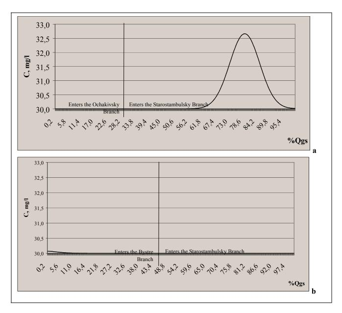
Figure 3. Concentration Ranges for Suspended Substances under Option 2 at the Gauging Stations No. 1 (a) and 2 (b)
